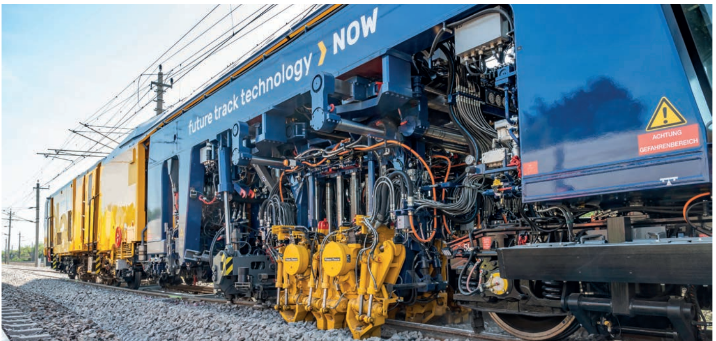
Fig 1. Electrically driven tamping machine with integrated ballast profiling and dynamic track stabilisation.
