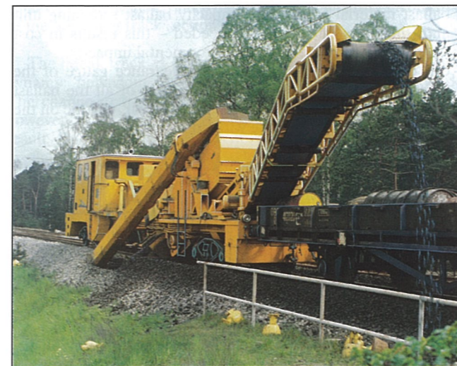
Fig. 6: The first fully hydraulic ballast cleaning machine – the RM 61 – a technological milestone
