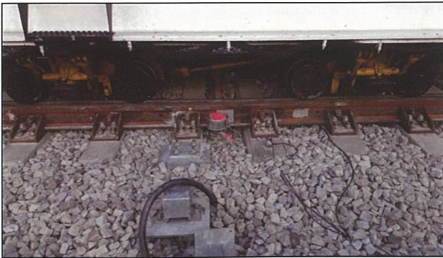
Fig. 3: Investigation into dynamic track stabilisation in France [5]
