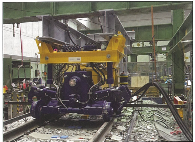
Fig. 4: DTS experiment at the test laboratory of TU Munich, Germany
