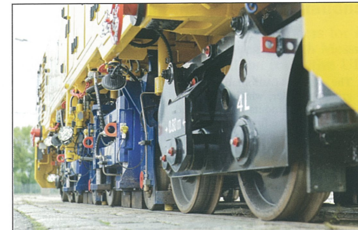
Fig. 3: The grinding units of the ATMO oscillating rail grinding trailer
