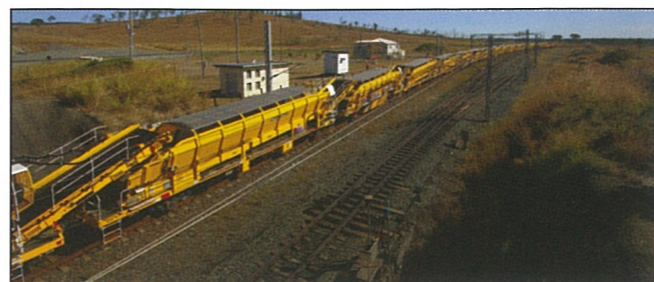
Fig. 4: MFS units – efficiency in spoil logistics
