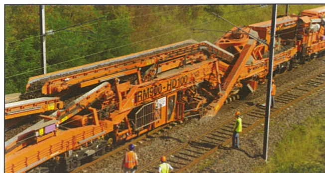
Fig. 7: The RM 900 HD high-output ballast cleaning machine with two screening units and integrated supply of new ballast
