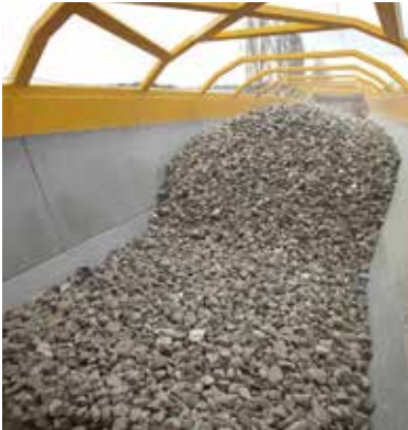
Integrated hopper units during track maintenance are a contribution to the goal of major railways: to achieve a closed loop economy
