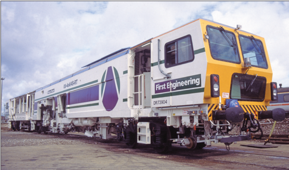
Above: First Engineering's Plasser & Theurer 08-4x4/4S-RT Unimat tamper was the first post-privatisation on-track machine to be delivered to a UK contractor in 1997. It also heralded the introduction of a new generation of machines to the country that were designed and constructed to the then new Railway Group Standards. Photograph: Alex Hall.
