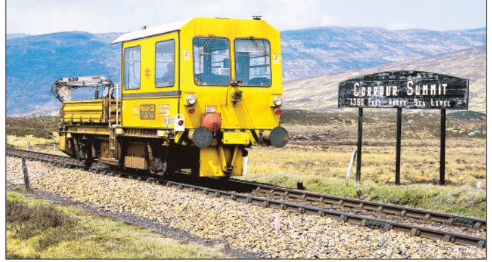
Above: Machines for general infrastructure maintenance have also been manufactured by Plasser & Theurer, such as this TASC-45 pictured at Corrou Summit. Photograph: NPT Publishing Collection.
