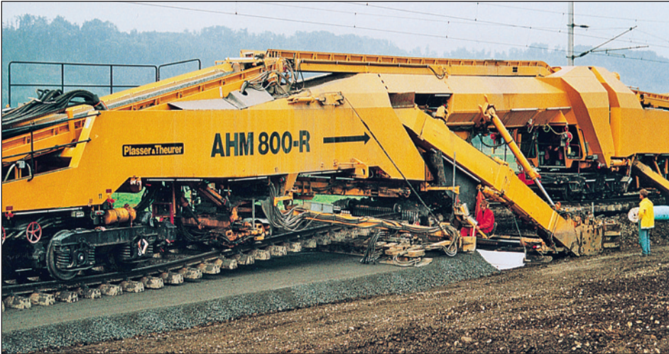
Above: In 1996, the AHM 800-R was developed by Plasser & Theurer as a combined track formation rehabilitation and ballast cleaning machine. Photograph: Plasser & Theurer.
