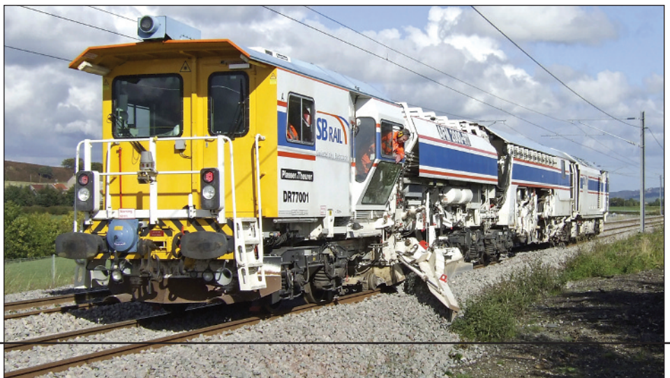
Above: First Engineering's Plasser & Theurer 08-4x4/4S-RT Unimat tamper was the first post-privatisation on-track machine to be delivered to a UK contractor in 1997. It also heralded the introduction of a new generation of machines to the country that were designed and constructed to the then new Railway Group Standards. Photograph: Alex Hall.
