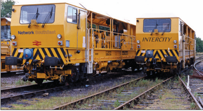
Above: The development of Dynamic Track Stabilising (DTS) technology led to the delivery of a fleet of DTS machines to British Rail during 1987 and 1988. Photograph: Roy Hennefer.
