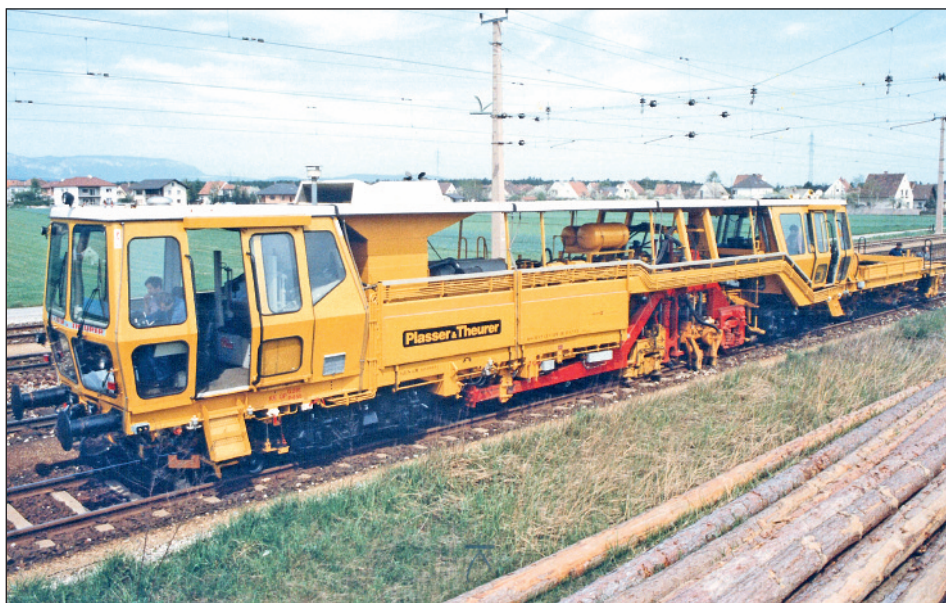
Left: In 1983, the first levelling, lining and tamping machine to work continuously - the 09-CSM - was developed by Plasser & Theurer. Photograph: Plasser & Theurer.
