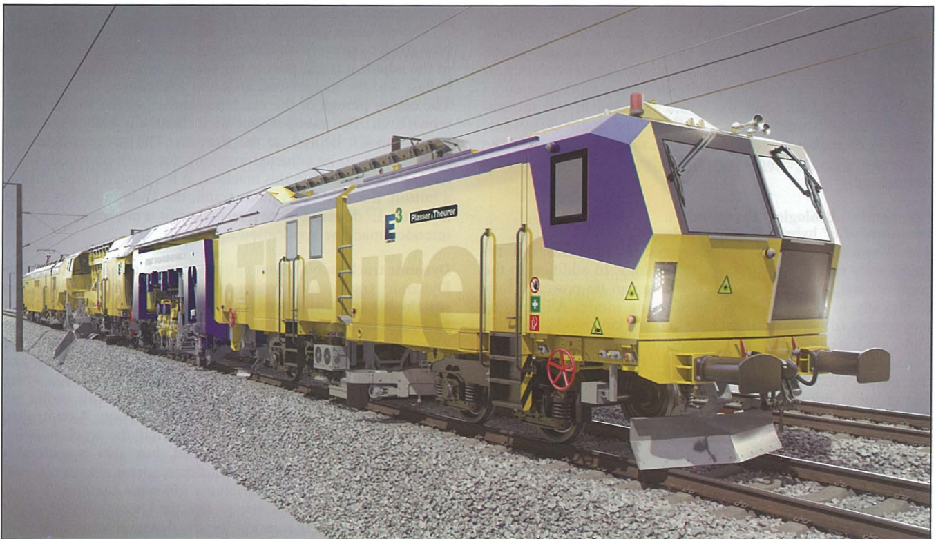
Fig. 1: The new Unimat 09-8x4/4S BR Dynamic E 3 : ballasting, tamping, profiling, stabilising, surveying, as well as pre- and post-measuring – all performed by a single machine
