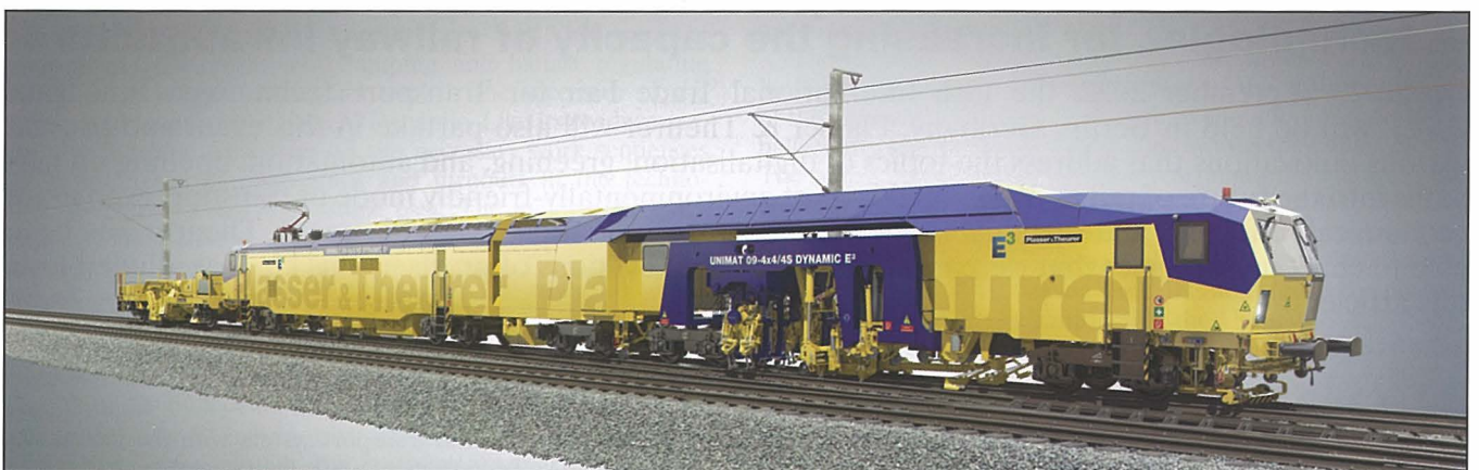
The Unimat 09-4x4/4S Dynamic E 3 with hybrid drive technology
