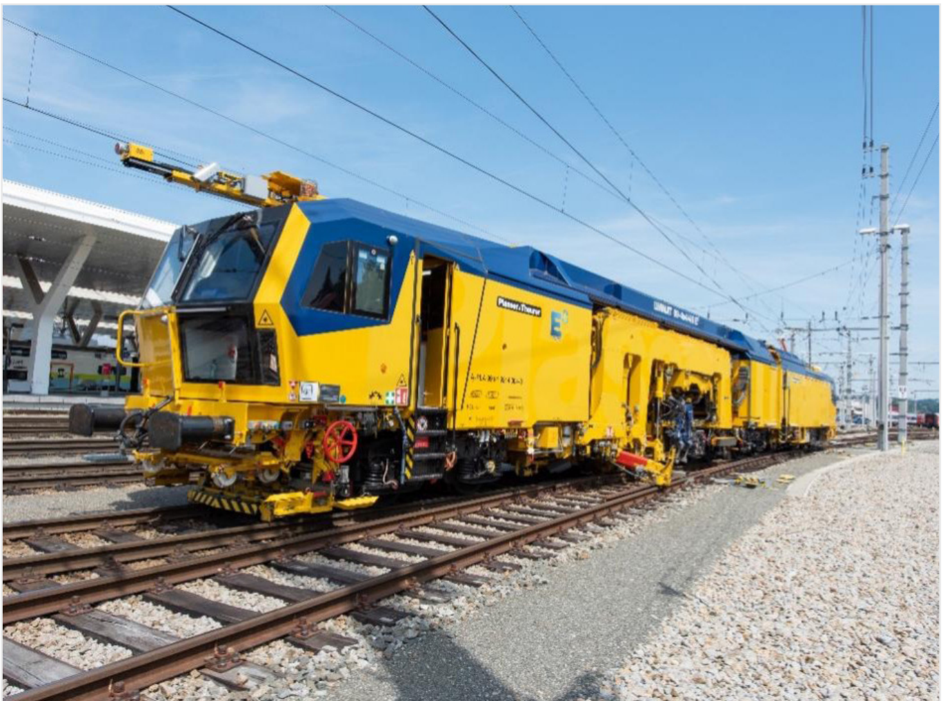
Figure 1: Tamping machine equipped with PlasserSmartTamping - The Assistant [4].
