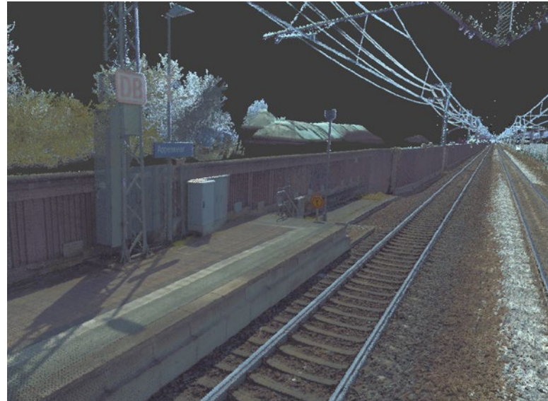
3: Colored point cloud from the Offenburger Tunnel project
